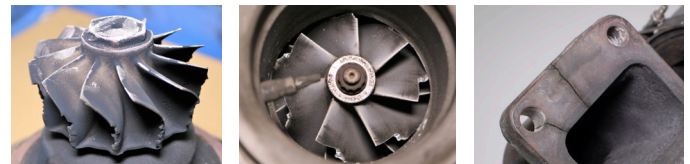
Damaged Turbine Wheel
